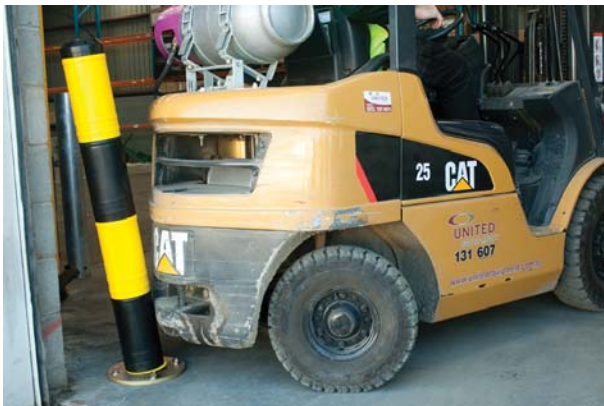
SABs protect against damage by simply absorbing this kind of impact.
