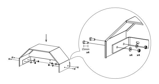
mudguard to chassis \_\_\_\_\_
