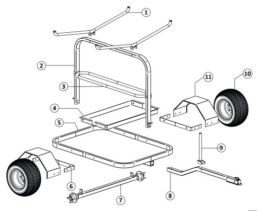
tray and axle assembly \_\_\_\_\_
