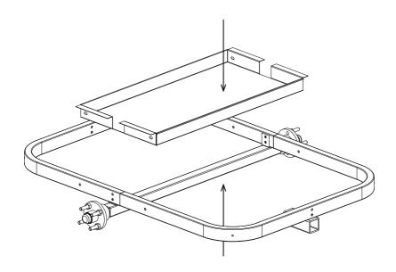
mudguard assembly \_\_\_\_
